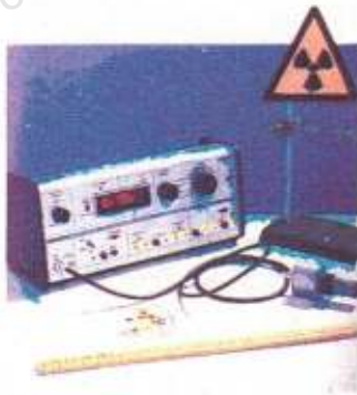
(b) G.M. Tube with scaler unit Fig. 21.9
