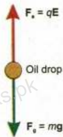
Fig. 12.23 (b) Oil drop balanced by the gravitational force and the Coulomb force.
