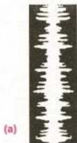
Fig 19.8 Sound track on a film which varies the intensity of light reaching the photo cell.
