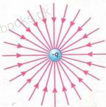
Fig. 12.7 The electric field lines are directed radially inward towards a negative point charge -q .
