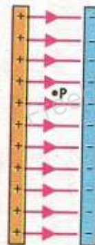
Fig. 12.19 The lines of force between the plates are normal to the plates and are directed from the positive plate towards the negative one.
