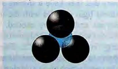
Fig (4.22 c) The formation of a tetrahedral site, due to four balls
