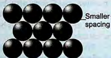
Fig (4.22 b) Packing of eleven spheres in a box (two dimensional view)
