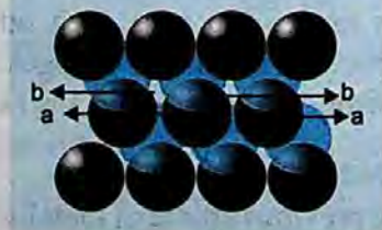
Fig (4.22 d) Close packing of spheres, showing 11 balls in first layer and 6 balls in second layer
